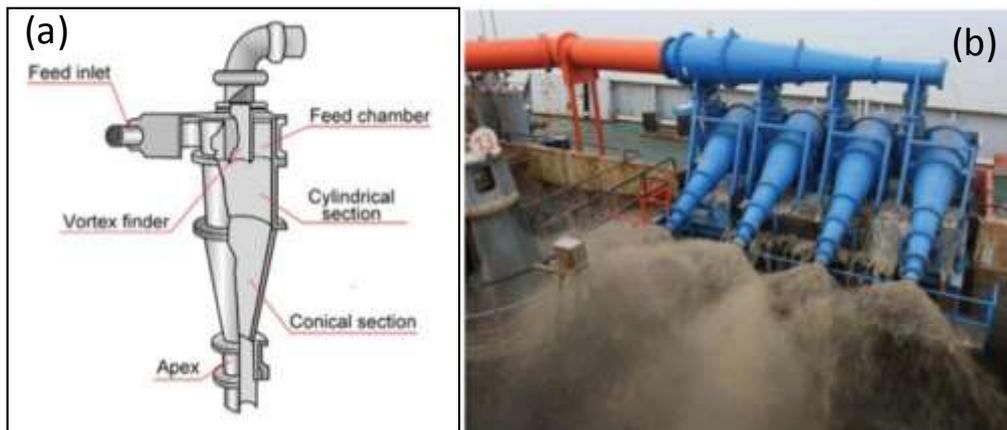
**Figure 1.2:** Cyclone classifiers: (a) Cross-sectional view (Wills & Finch, 2016); (b) Cyclone particle classifiers in operation ([www.dredgingtoday.com](http://www.dredgingtoday.com)).
