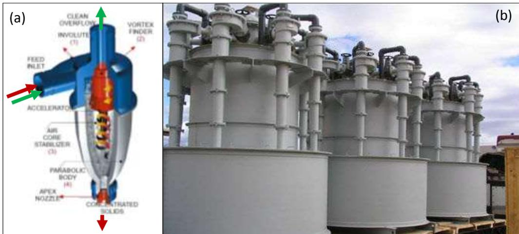
**Figure 1.1:** (a) A sectioned hydrocyclone particle classifier ([www.oilfied.gnsolids.com](http://www.oilfied.gnsolids.com));(b) A cluster of hydrocyclones used in a Metallurgical plant connected in series ([www.flsmidth.com](http://www.flsmidth.com)).
